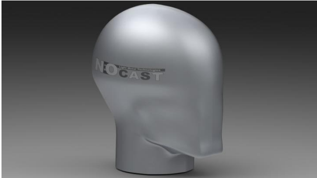
Fig. 1. Type 625 magnesium alloy headform that includes a base for attaching a 7265A-type sensor
